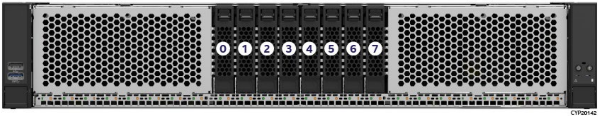
Figure 24. 2U 8 x 2.5" Front Drive Bay Configuration – M50CYP2UR208
