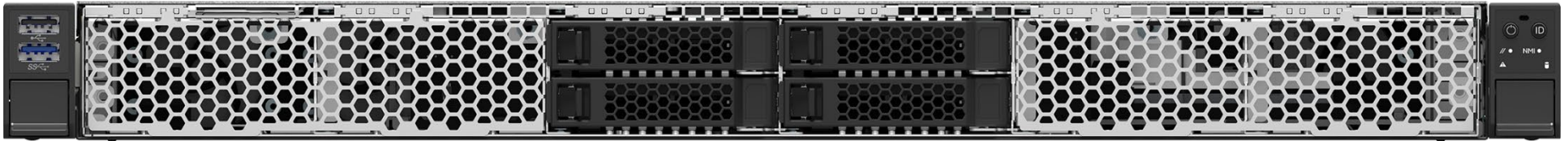
Figure 6. 4 x 2.5" front Drive Bay Configuration – M50CYP1UR204
